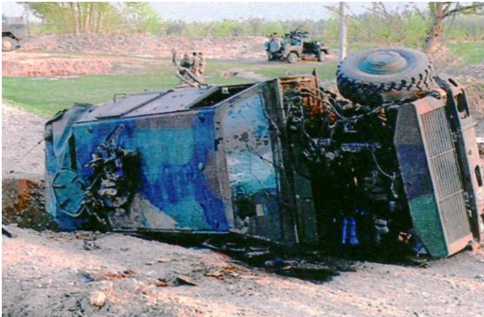
German Army DINGO II in Afghanistan after heavy mine attack; without Explosion or fire
